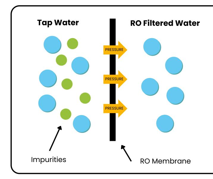
High-pressure forces water through the semipermeable reverse osmosis membrane element. RO membranes are made of a thick polyamide file that contains tiny pores through which water can flow.
