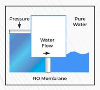
High pressure forces water through the semipermeable reverse osmosis membrane element. RO membranes are made of a thick polyamide file that contains tiny pores through which water can flow.
